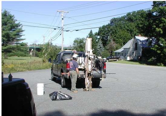
Sampling to determine current soil and groundwater quality.
