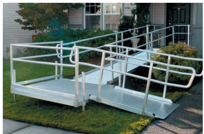
Ramps built out of no-contextual materials stick out and detract from the curb appeal of a house, especially when they project out in front of the building.
