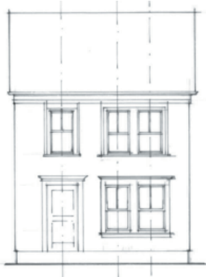
Windows usually stack to maintain the structural integrity of the load-bearing walls, which transfer structural loads down between the openings.
