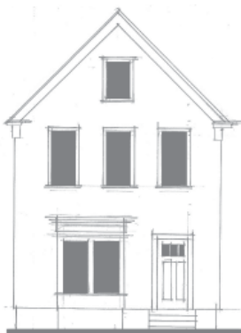
Use vertical proportions generally. Avoid horizontal windows unless they are composed of groups of square or vertical windows.
