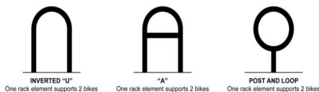
Figure 7. One Rack Bicycle Rack Examples Source: RPTA/Valley Metro: Bus Stop Program and Standards
