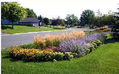
Water enters the rain garden, then dissipates slowly into the ground
